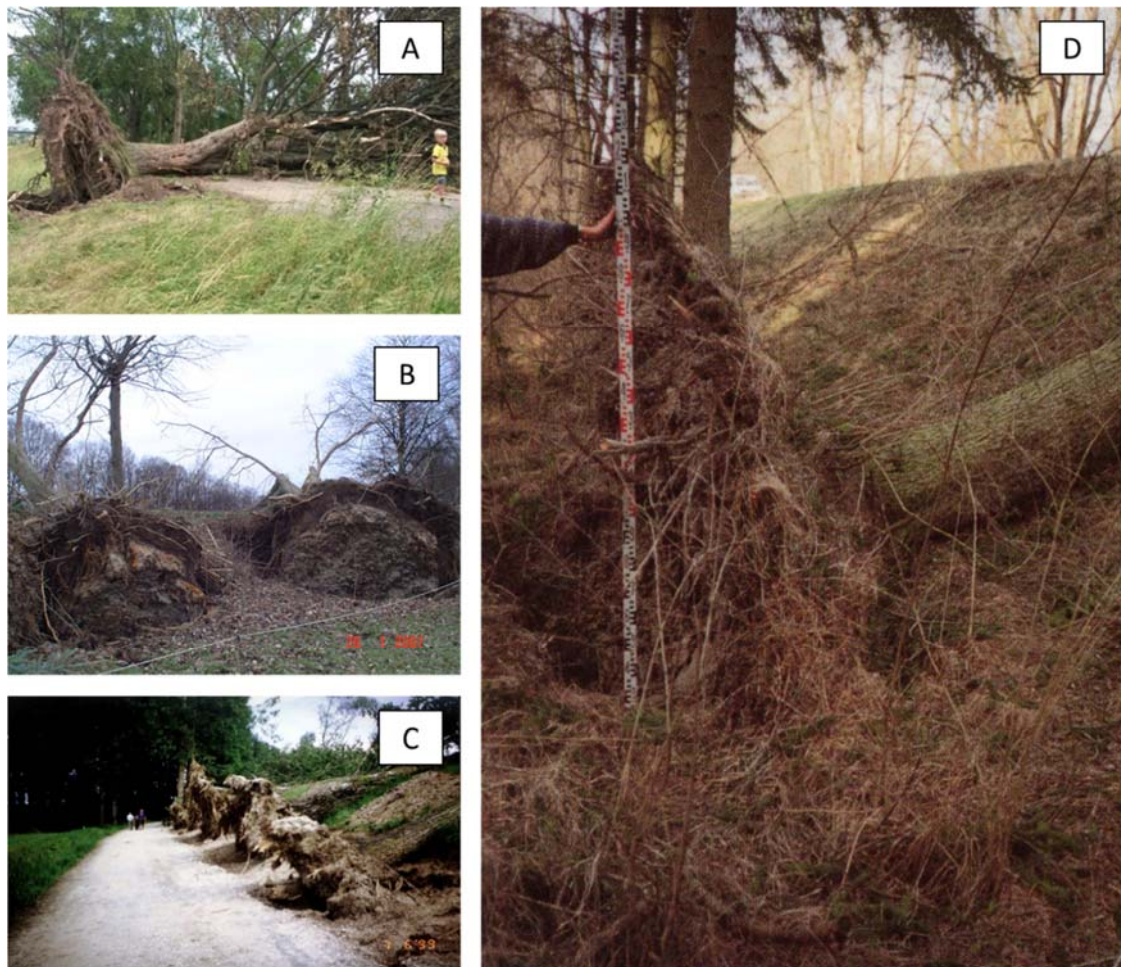
Figure 6: Selected tree failures by windthrow at levees in Germany (A: windthrow at a Rhine levee during the storm Ela 2014 in Duesseldorf, Source: SEBD / B: windthrow at levees with the Black Magpie during storm Kyrill 2007, Source: LUA Brandenburg / C: thrown row of poplars at the landside levee toe in 1999, Source: StMUVG / D: Thrown spruce at the landside levee toe at the river Lech in Bavaria, Source: LfW BY 1990)
