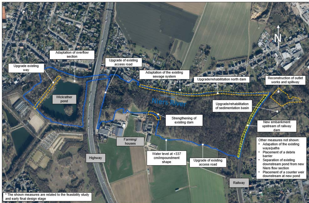
Fig. 2. Plan view of the complete reservoir with planned measures and the reservoir water level at +3,37 m above reservoir gauge zero-point
