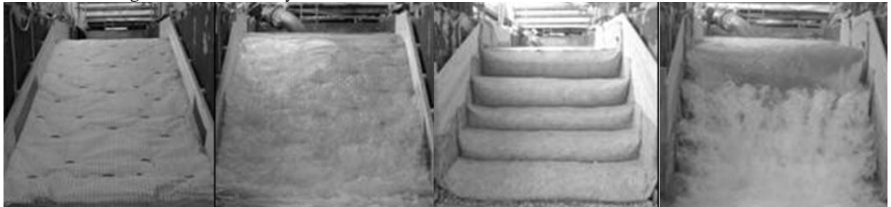
Figure 5. Loaded and unloaded dike models with slope parallel geosynthetic layers using anchors for fixation (left) and horizontal, folded layers (loops) (right) (Haselsteiner et al. 2007a, b)
